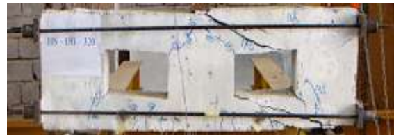
Figure 14: Crack pattern at ultimate load for beam HS-DB-320 (Group B) (diagonal splitting failure)
