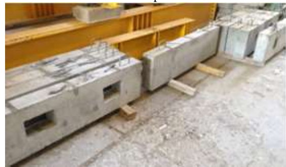
Figure 6: Tested deep beams after completing casting and curing process
