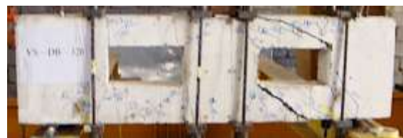
Figure 17: Crack pattern at ultimate load for beam VS-DB-320 (Group B) (shear – compression failure)
