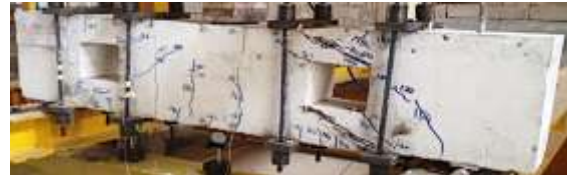
Figure 15: Crack pattern at ultimate load for beam VS-DB-160 (Group C) (shear – compression failure)
