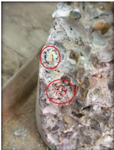
Picture (4): balls after curing and tests of water absorption polymer (WAP) mixes
