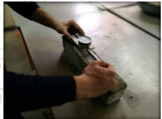
Picture (2): measuring volumetric change by extensometer device
