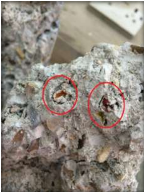
Picture (3): water absorption polymer balls exploded in concrete
