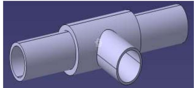
Figure 9: Modeling the Dn 63 mm T-type branch tee
