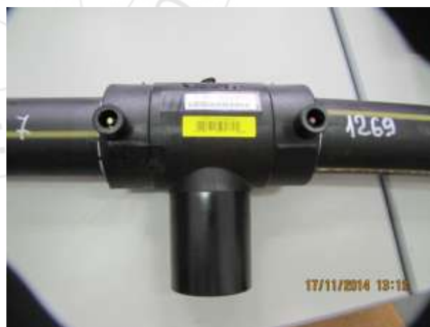
Figure 5: Equal tee - polyethylene pipe Dn63 assembly resulting from electro-fusion welding
