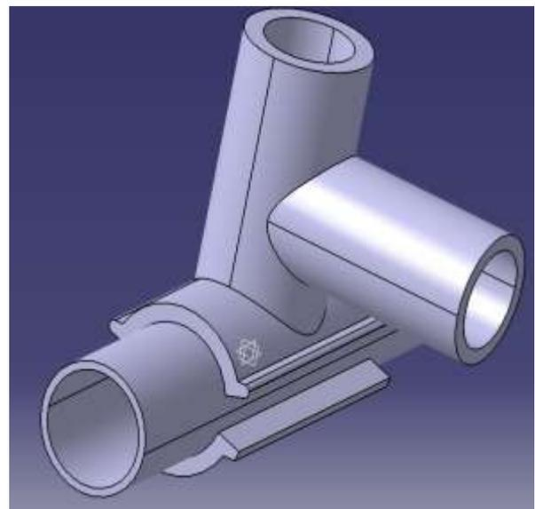
Figure 10: Modeling the Dn 63 mm branch tee
