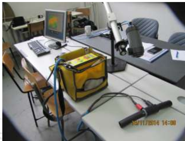
Figure 4: Welding machine and temperature measuring system
