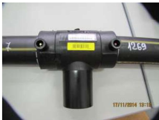
Figure 5: Equal tee - polyethylene pipe Dn63 assembly resulting from electro-fusion welding
