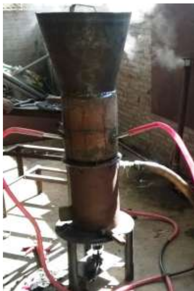
Figure 1: Gasifier Developed at Laboratory based on the CAD Model
