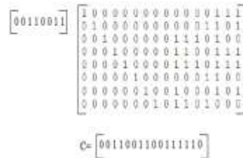
Figure 5.8: Encoding of Regular Parity Matrix2
