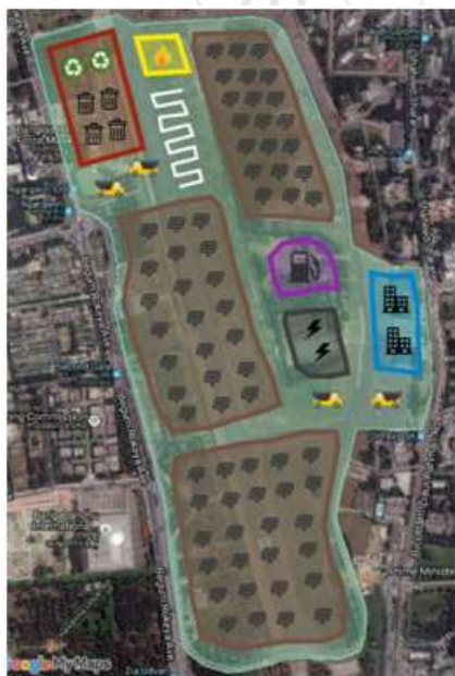
Figure 1: Conceptual design of the urban solid waste management facility, with landfills, photovoltaic panels, incinerator and establishments on site created using Google My-Maps.
