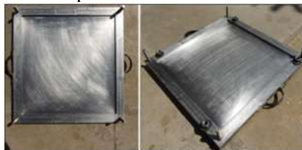
Figure 3.2.1: Mold bottom after machining and finishing operations.
