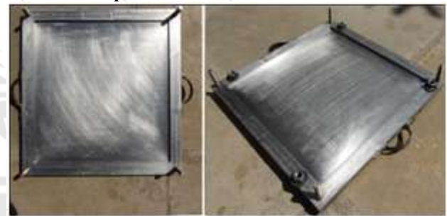
Figure 3.2.1: Mold bottom after machining and finishing operations.
