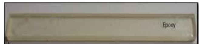
Figure 4: Photograph of Flexure Test Specimen for pure epoxy.
