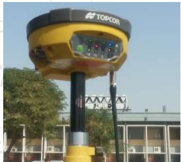
Figure 2: The HiPer II receiver in the work field
