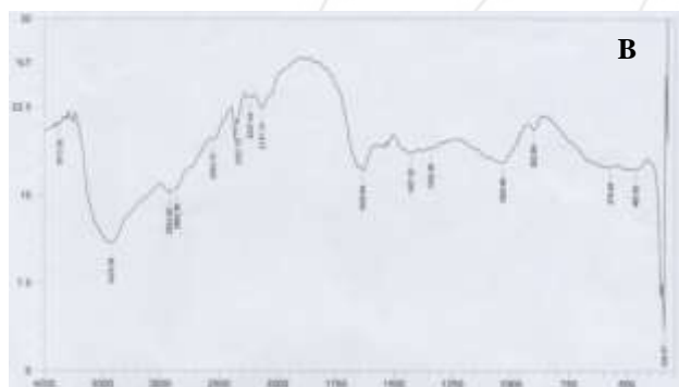
Figure 2: FTIR test results of bacterial cellulose produced by Gluconacetobacter xylinus at (A) 23 °C (B) 30 °C
