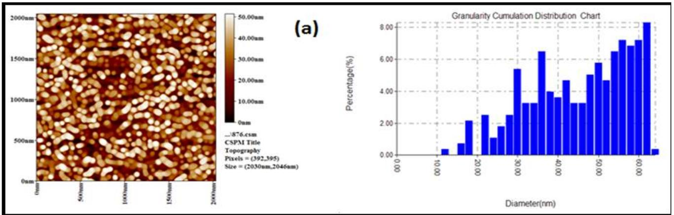
Figure 7: (2D) image and histogram of TiO<sub>2</sub> / ZnO (100/0 %)
