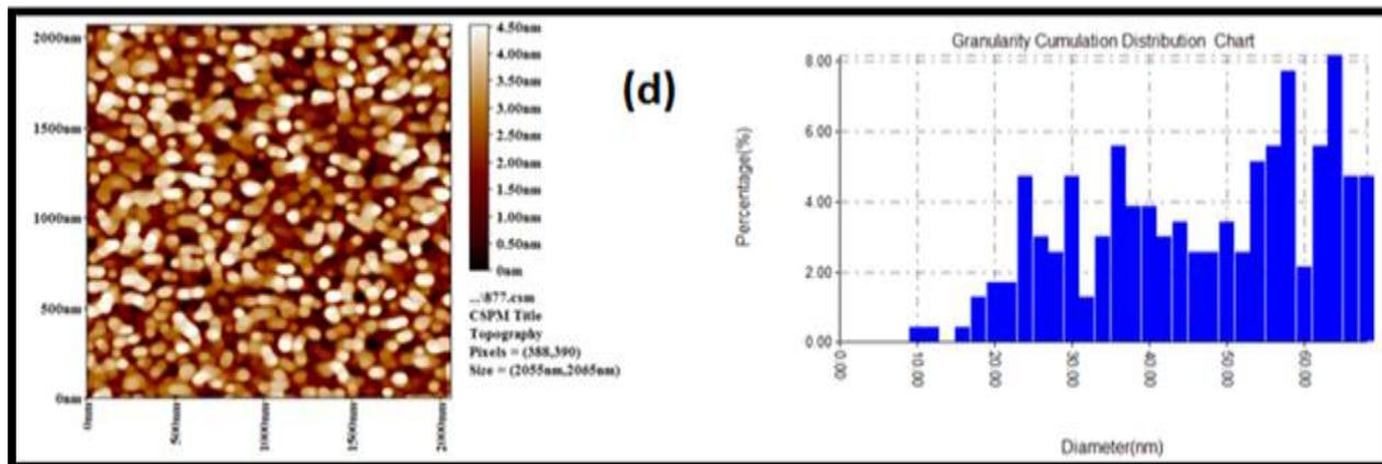
Figure 10: (2D) image and histogram of TiO<sub>2</sub> / ZnO (50 % / 50 %)
