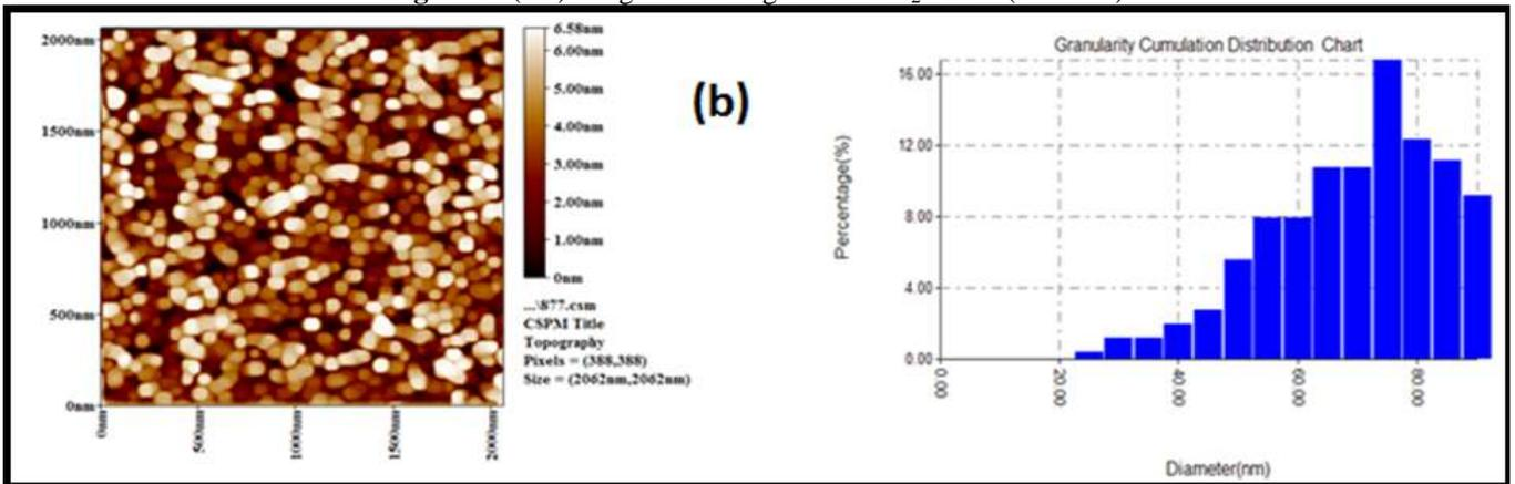
Figure 8: (2D) image and histogram of TiO<sub>2</sub> / ZnO (0% /100 %)
