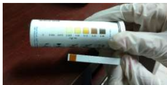
Figure 2: Testing of arsenic kit with a standard solution of 200 ug/L
