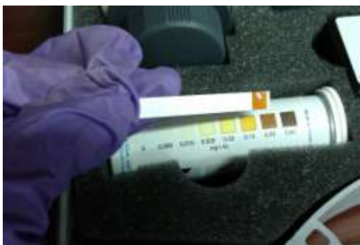
Figure 6: Result for an arsenic solution with As:Fe ratio 1:5 left for 18 hours
