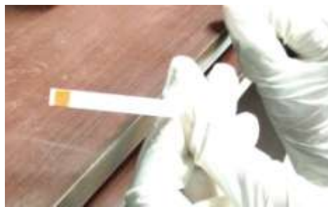
Figure 9: Result for arsenic solution with As:Fe ratio of 1:20 and pH 7
