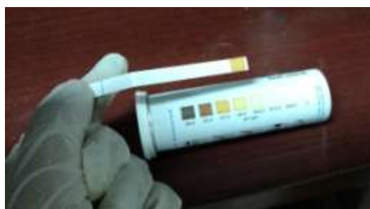
Figure 10: Result for arsenic solution with As:Fe ratio of 1:20 and pH 6
