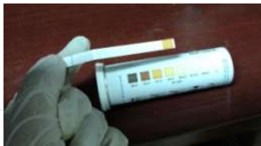
Figure 10: Result for arsenic solution with As:Fe ratio of 1:20 and pH 6
