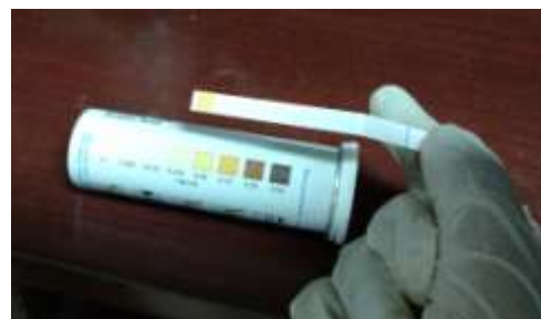
Figure 1: Testing of arsenic kit with a standard solution of 40 ug/L
