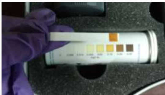
Figure 7: Result for an arsenic solution with As:Fe ratio 1:5 in absence of sand-bed
