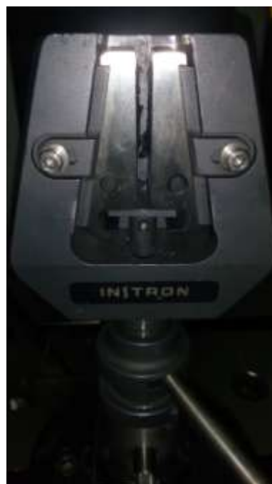
Figure 7: Clamp used for fixing the specimens
