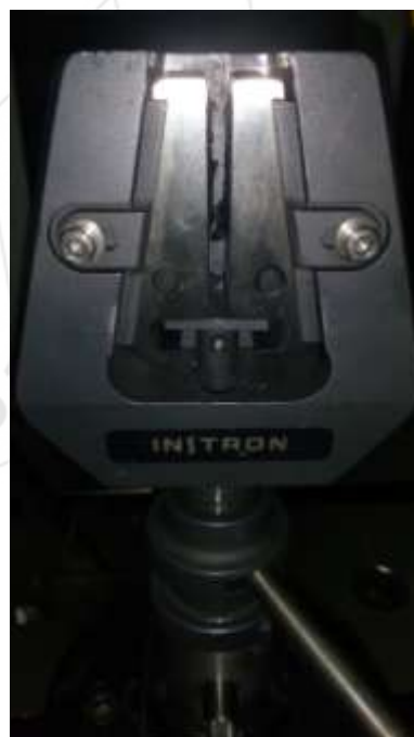
Figure 7: Clamp used for fixing the specimens
