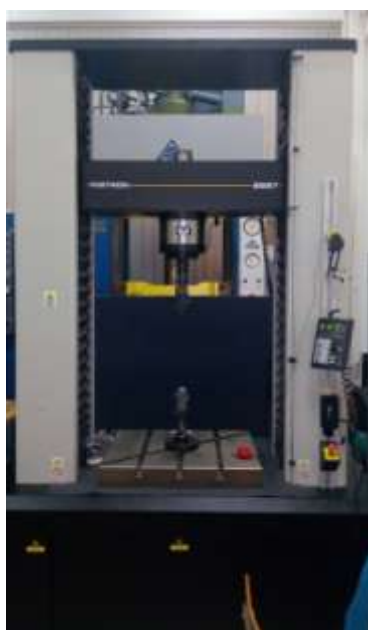
Figure 6: Instron traction testing machine with the Aramis optical measuring system
