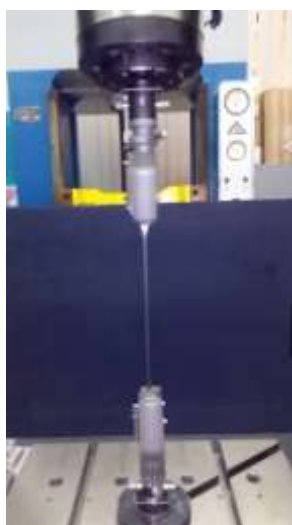
Figure 8: The uniaxial tensile testing of polyethylene without stress concentrators
