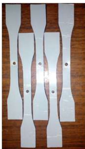
Figure 9: Polyethylene specimens with defect simulation
