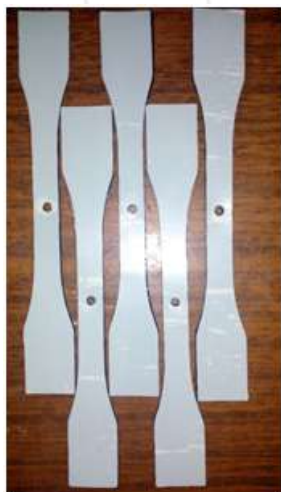
Figure 9: Polyethylene specimens with defect simulation
