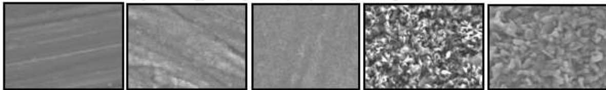
Figure 1: Surface topography for test groups I, II, III, IV, and V from left to right (SEM mag. 10 kx).
