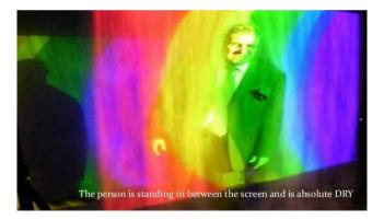
FogScreen creates a dry fog by ensuring that the water droplets are in the range of 2-3 microns in size and are electro statistically charged so that they move around and away from other objects.
