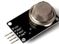
Figure 4: MQ135 (Gas Sensor)[4]
