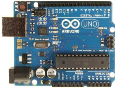
Figure 2: Arduino uno board[1]
