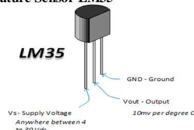
Figure 6: Temp Sensor LM-35[6]
