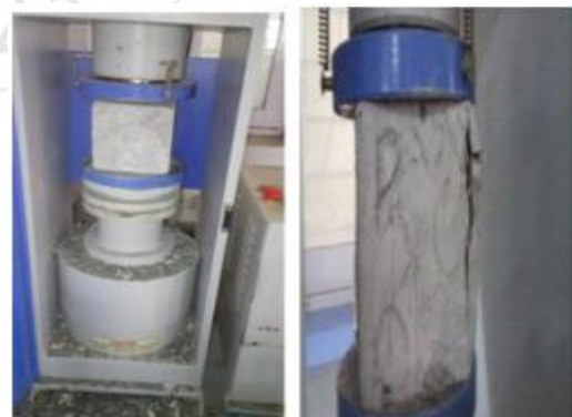
Figure 4: Testing of cubes in compressive testing machine
