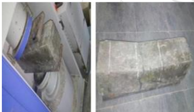
Figure 6: Testing of Beams in Flexural Testing Machine
