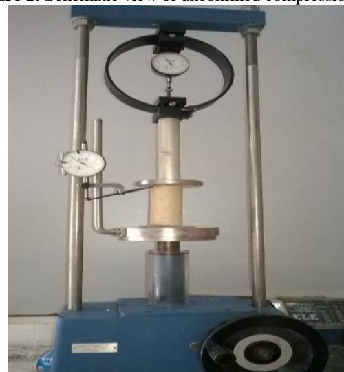
Figure 2: Unconfined compression test machine
