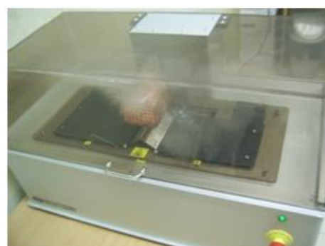
Figure 5: The thermocycling device
