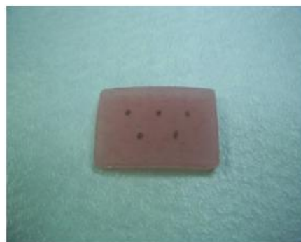
Figure 4: A test sample with indentations for measurement
