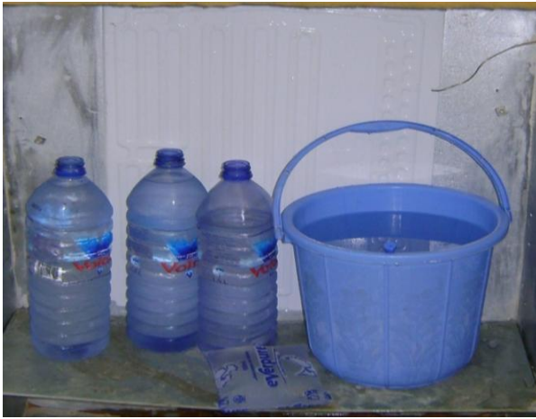
Figure 5 (d): set up for taking the temperature of the water to be cooled in both the normal and the dual purposed refrigerators
