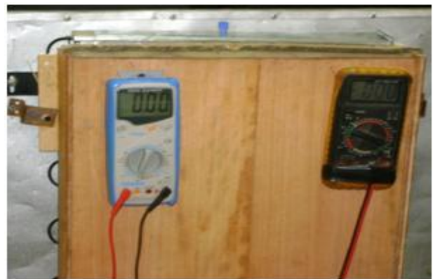
Figure 5 (a): set up for taking the temperatures of the water in the tank.
