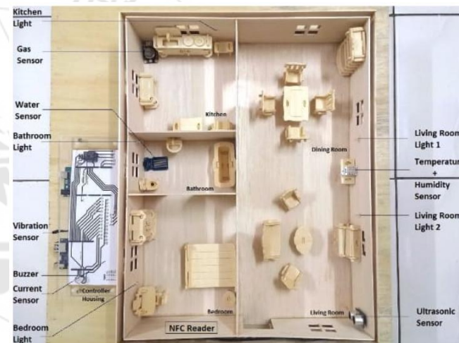
Figure 3: Structure of Home Security System [14]
