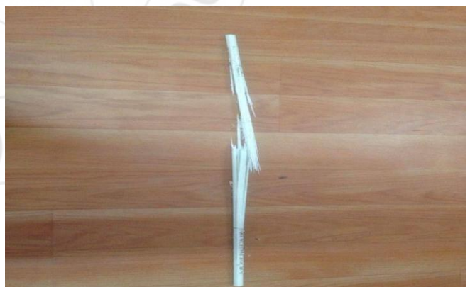
Figure 2: Tensile test on GFRP bar
