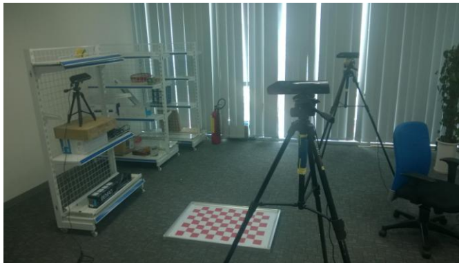
Figure 3: Setup Kinects around measurement area
