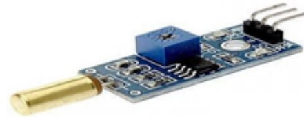
Figure 3: Tilt sensor module
