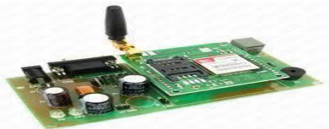
Figure 5: GSM system module
