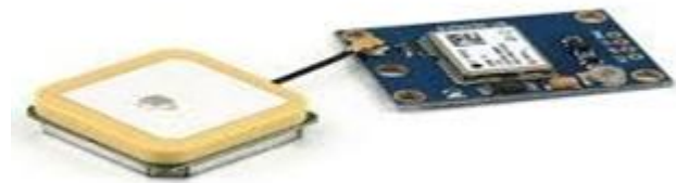
Figure 4: Global positioning system (GPS) module
