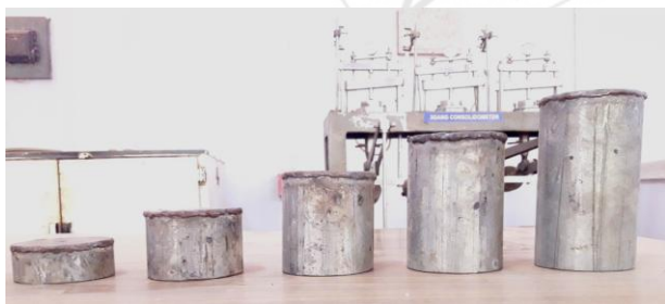
Figure 1 Model skirt footings
