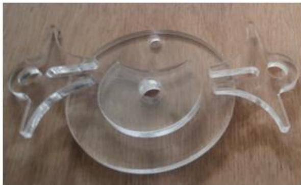
**Figure 4.1:** Driving wheel and driven wheel segments
