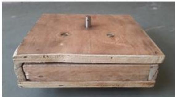
**Figure 4.3:** Wooden box with input or driving shaft on the top and two driven shafts at the bottom
