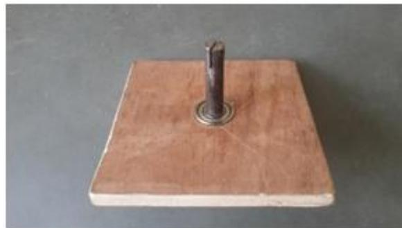
**Figure 4.5:** Supporting plates for wiper shafts
