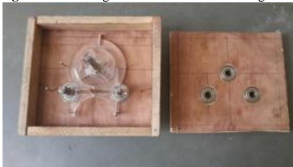
**Figure 4.2:** Modified Geneva mechanism in wooden box
