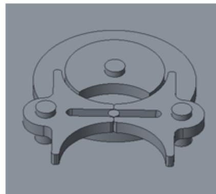
**Figure 3.1.2.1:** CREO model of modified Geneva mechanism
