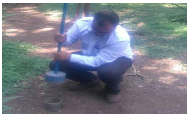
Figure 2: Sampling of Soil with Core cutter from field
