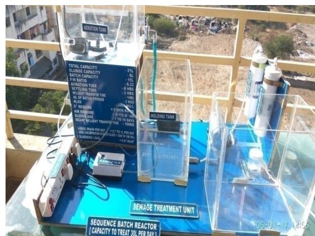
Figure 2: Pilot plant SBR Model
