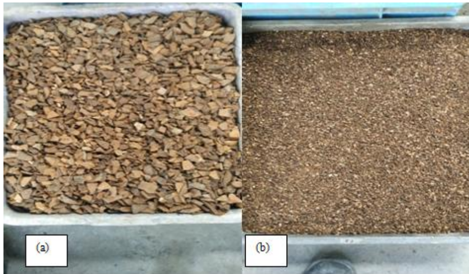
Figure 1: Crushed coconut shell aggregates (a) Coarse aggregate (b) Fine aggregate
