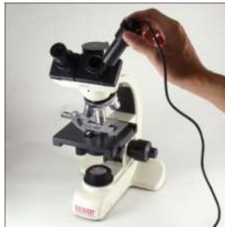
Figure 4: CMOS Camera attached with Microscope
