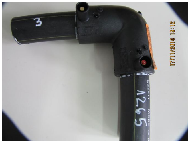
Figure 12: Polyethylene elbow - pipe assembly
