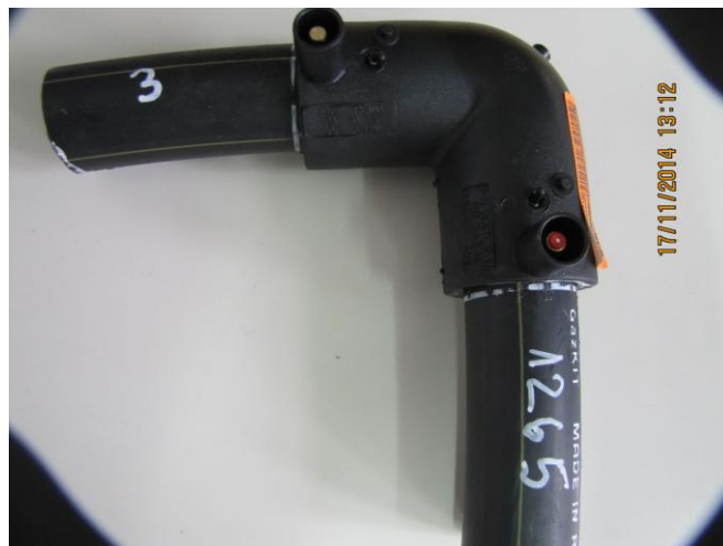
Figure 12: Polyethylene elbow - pipe assembly
