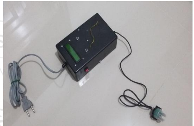
Figure 3.1: Prototype of Water Turbidity Measuring Device
