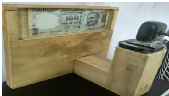
Figure 4: Camera and Stand used for Accessing the Currency and Colored object
