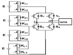
The more of the cascaded cells, the more voltage levels at the output side, and the output voltage is closer to the ideal sinusoidal. The dv/dt and the harmonics are very little. So it is a suitable topology for the energy storage system in electric vehicles and power grid
