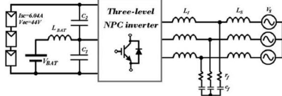
**Figure 5:** above shows the block diagram of simulation system.
