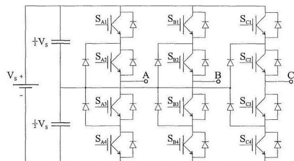
Figure 1: Three-level neutral point clamped inverter
