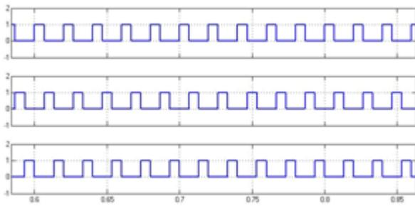
**Figure 7 (b):** Switching pulse for M1, M3, M5
