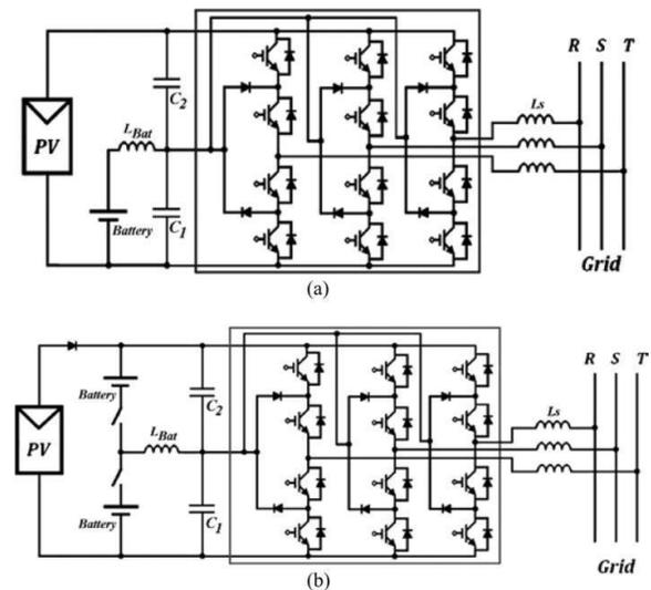
**Figure 4:** Proposed configurations for integrating solar PV and battery storage: (a) basic configuration; (b) improved configuration.
