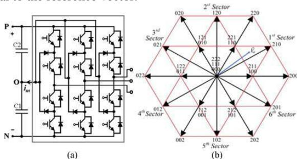
**Figure 3:** Typical three-level inverter (a) structure of circuit, and (b) three-level inverter space vector diagram
