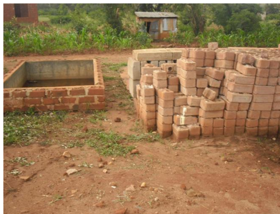
Figure 3: Locally produced burnt bricks in Morogoro town
