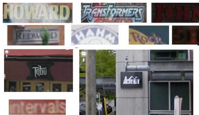
Figure 1: Some scene text images from ICDAR 2003 [2] and SVT [3]. The characters in these images have different fonts, shadows, distortions, deformations, low resolutions, and occlusions
