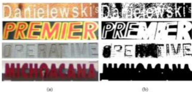
Fig. 3. The binarization results are quite disappointing, making it difficult for the following segmentation and recognition. (a) Scene text images. (b) Binarization result.
