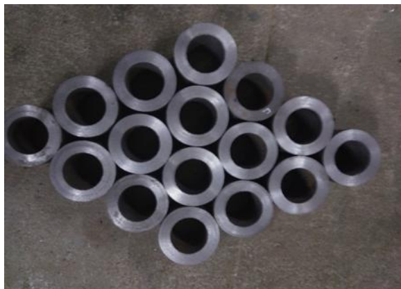
Figure 1: work material (ASTM A48 grey cast iron)
