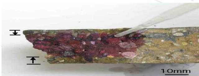
Figure 4: Phenolphthalein indicator solution applied to a fresh fracture surface through a concrete slab.
