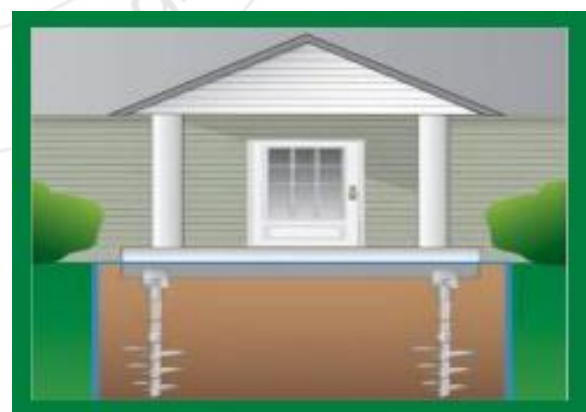
Figure 8: Ground Anchoring of the soil underneath foundation
