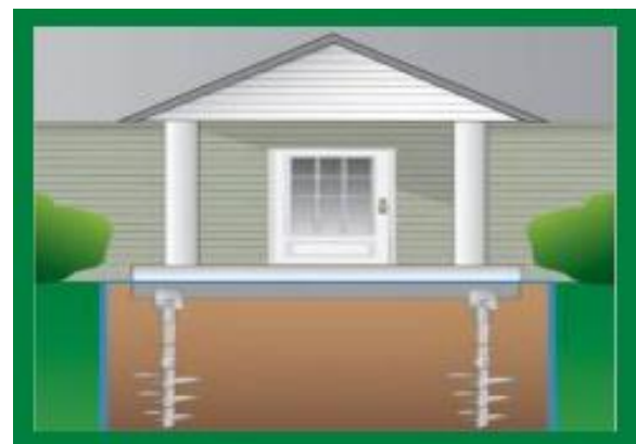
Figure 8: Ground Anchoring of the soil underneath foundation
