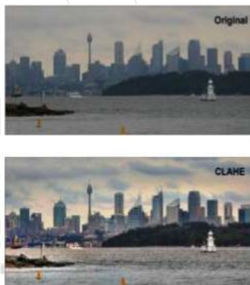
Figure 4: Original Image and Image Enhanced by CLAHE.
