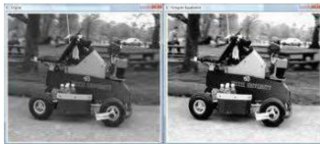
(a) Original Image (b) Enhanced image for Histogram Equalization
