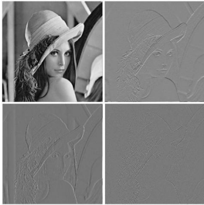
Figure 2: level 1 Redundant Discrete Wavelet Transform of an Image.
