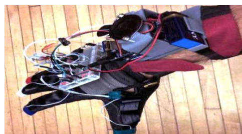
Figure 2: Glove based recognition system
