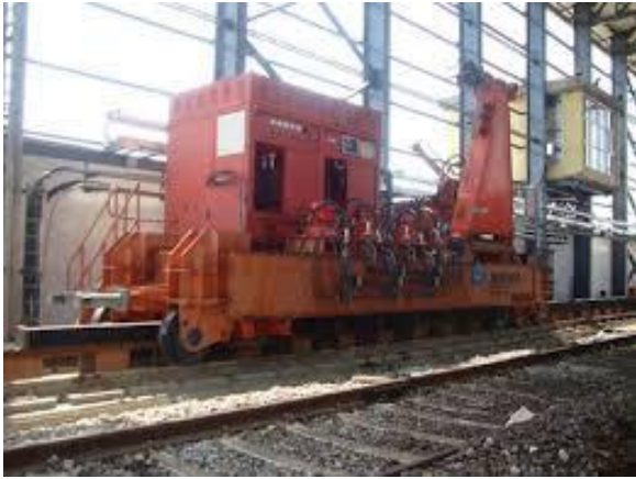
Figure 4: Side Arm Charger Equipment
