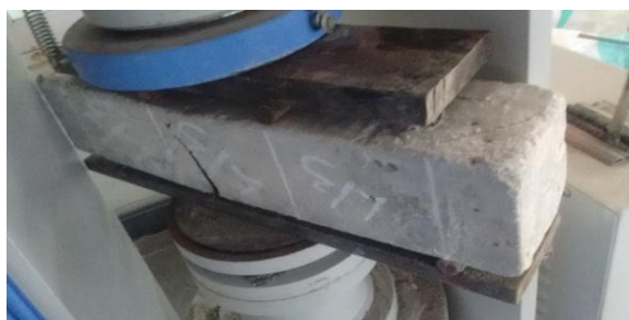
Figure 4: Flexural testing of beam
