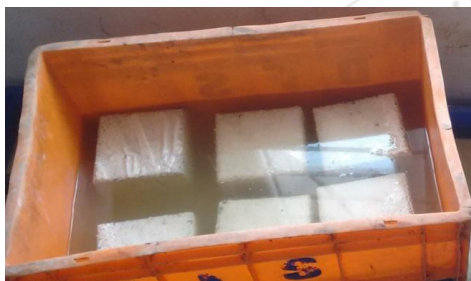
Figure 11: Curing of Cubes in H_2SO_4
