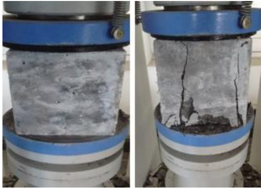
Figure 2: Compression testing of cube
