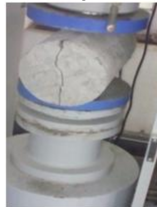
Figure 4(b): Testing of cylinders in compressive testing machine
