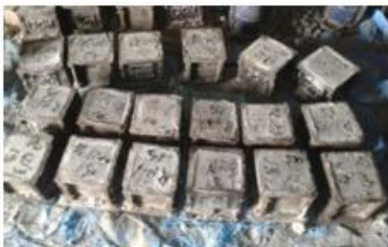
Figure 3(a): showing cubes compacted with concrete
