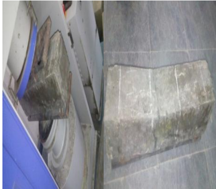
Figure 4(c): testing of beams in flexural testing machine
