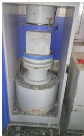
Figure 5: Cubes for compression testing
