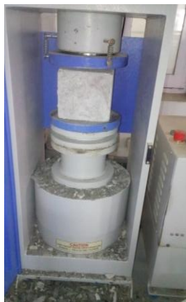
Figure 5: Cubes for compression testing
