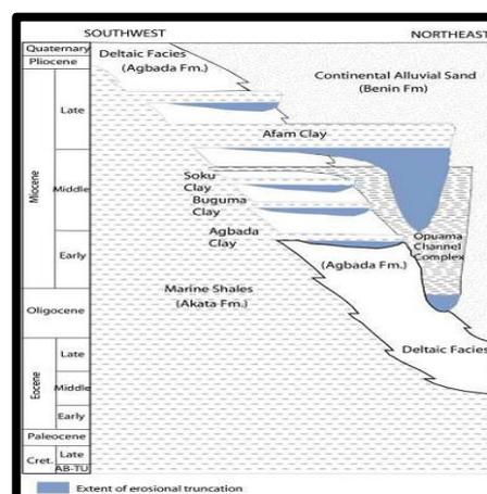
**Figure 2:** Stratigraphic column showing formations of the Niger delta (modified from [8] and [13]).
