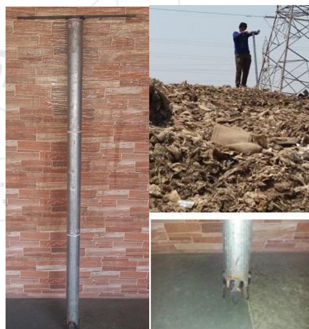
Figure 1 (clockwise direction): a) Designed Sampler of 6 feet b) Site Photograph while taking sample c) bottom of sampler
